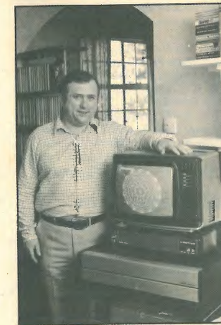
Mike Aldrich, managing director of Rediffusion Computers, with a Teleputer system, one of a range of videotex terminals that his firm believes will be at the centre of the 'home information system' towards the end of the 1980s. The terminals combine broadcast tv, videotex, video tape recorder, video disc and telecommunications with personal computers.
